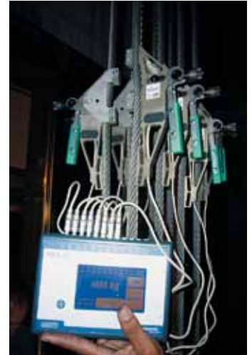
Fig. 38: Simultaneous measurement of rope tensile force
